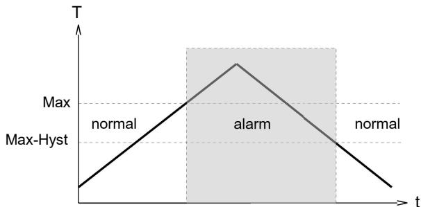
The change to the alarm state is indicated by the integrated red LED and a cleartext in the display.
