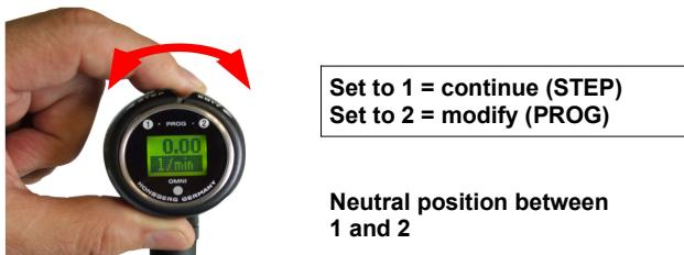
The ring can be removed to act as a key, or turned through 180 ° and replaced to create a programming protector.
