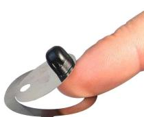
Because the diaphragm only bends, and functions without a bearing, there is almost no frictional effect. The movement therefore occurs practically free of hysteresis, and the test results have very good reproducibility.
